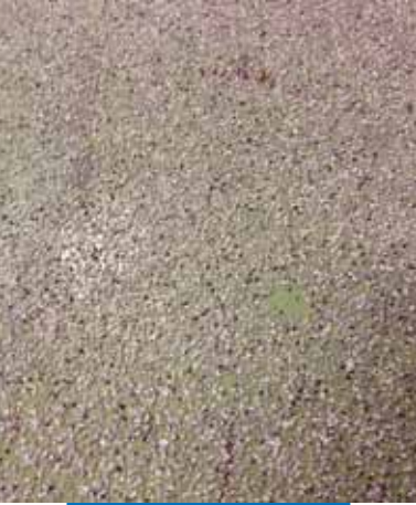
Compact method - primer scattered with Mapequarz color
